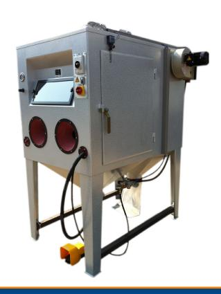
The Airblast Vacuum Injection Cabinets are designed for manual or automatic shotblasting of all sorts of smaller items. The general jobs done in these cabinets are delicate or lighter work, like: rust removal, cleaning, slagging, frosting, chipping and polishing.
