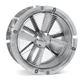
The Airblast Jet Fan is a four-bladed vaneaxial fan which operates through a highvelocity jet of compressed air which is ejected from the trailing edge of the blade. This results in the forward rotation of the fan wheel just like a jet plane is pushed forward by the high-velocity jet ejected from the rear of the jet engine.
