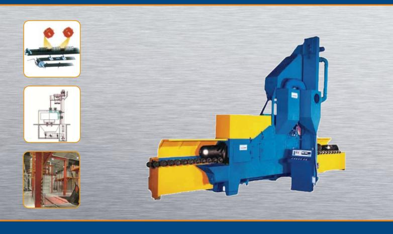
The AB265, AB2615, and the ABES1422 have been specifically designed to acheive the perfect result when blasting round springs. Round springs offer a unique blasting challenge - complete blasting coverage is vital in the critical environment in which the springs operate. Positioning of the blast wheels is crutial in achieving the desired result.
